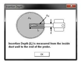
Figure 3-11. Insertion Depth diagram
