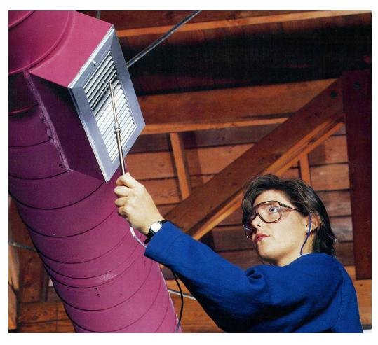
Kurz Portable Air Velocity Meters are used worldwide because of their accuracy and extremely fast flow response measurements in a variety of industrial applications. The constant power, thermal flow technolgy used for all Kurz instrumentation supports a direct mass flow reading and flawless repeatability.
